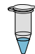
250 \mu l Buffer RS 250 \mu l Buffer LS 350 \mu l Buffer BS 12,000 rpm 离心 10 min 取上清
